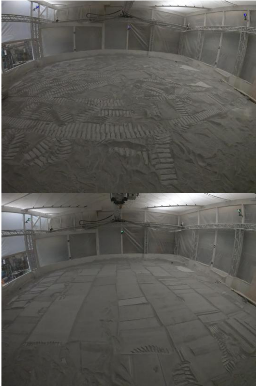
Figure 2: MLSS post infill(top), and post flattening (bottom) operations.
